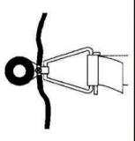
Make sure all insulators are closed and ground rods are connected properly. Turn on fence charger and check voltage at end of fence. Walk the fence to look for arcing, broken insulators, loose Pro-Tek tape or vegetation touching fence etc. Check voltage regularly. Use a low-impedance fence charger only.
